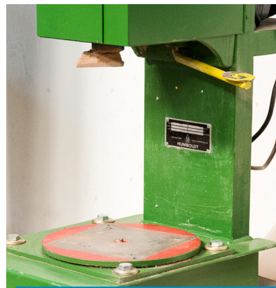
AUTO PROCTOR HAMMER FOR MOISTURE DENSITY RELATIONS
