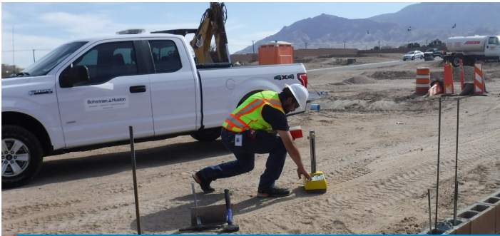
DENSITY AND MOISTURE TESTING FOR COMPACTION
