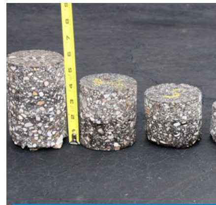
CORES FOR PAVEMENT THICKNESS VERIFICATION
