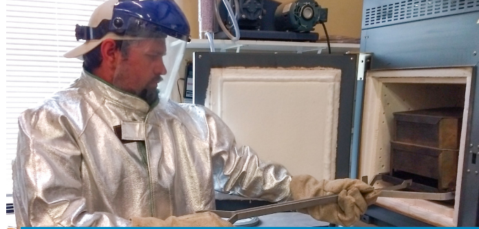
ASPHALT CONTENT TESTING BY IGNITION
