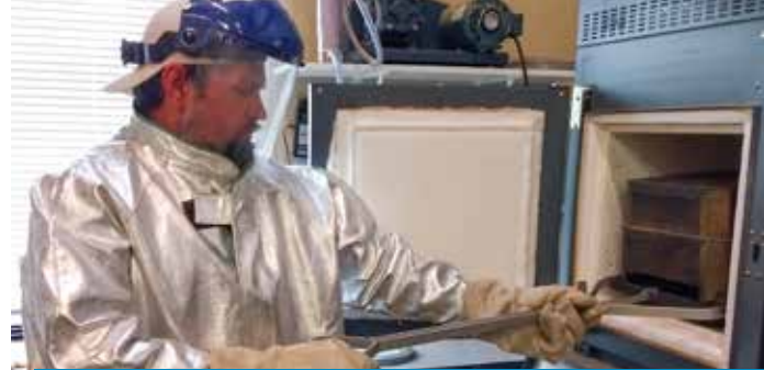
ASPHALT CONTENT TESTING BY IGNITION
